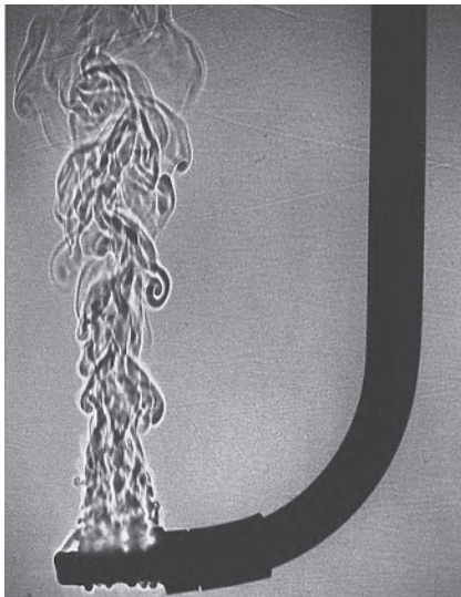
Figure 17.28 A heating element in the tip of this submerged tube warms the surrounding water, producing a complex pattern of free convection.
