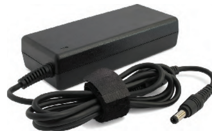
Figure 31.22 An ac adapter like this one converts household ac into low-voltage dc for use in electronic devices. It contains a step-down transformer to change the line voltage to a lower value, typically 3 to 12 V, as well as diodes to convert alternating current to the direct current that small electronic devices require (see Fig. 31.3).
