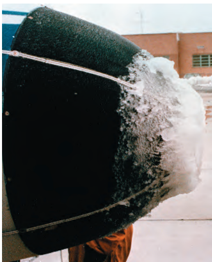
Figure 17.22 When this airplane flew into a cloud at a temperature just below freezing, the plane struck supercooled water droplets in the cloud that rapidly crystallized and formed ice on the plane's nose (shown here) and wings. Such in-flight icing can be extremely hazardous, which is why commercial airliners are equipped with devices to remove ice.
