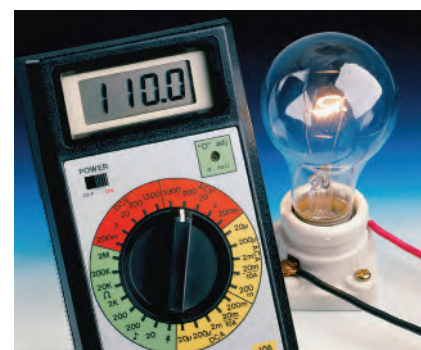
Figure 26.18 This digital multimeter can be used as a voltmeter (red arc), ammeter (yellow arc), or ohmmeter (green arc).
